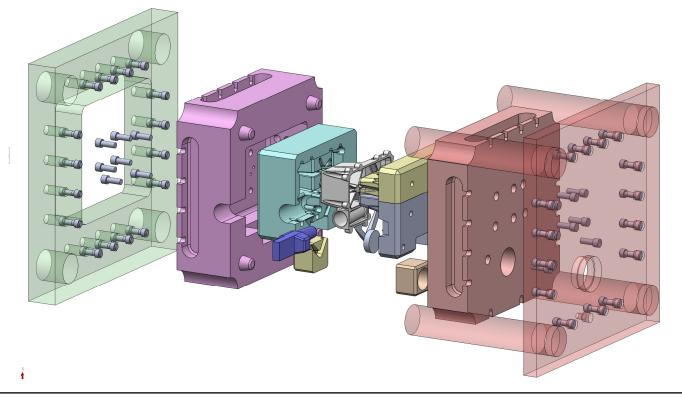
A simple set of cooling loops is cut into the model cavity inserts.
