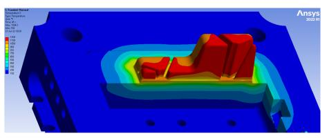
Of particular interest are temperatures in the cover side inserts. The deep pocket in the part translate into isolated towers in the mold shape. These towers can get very hot, leading to temperature imbalance with the bulk material of the insert.
