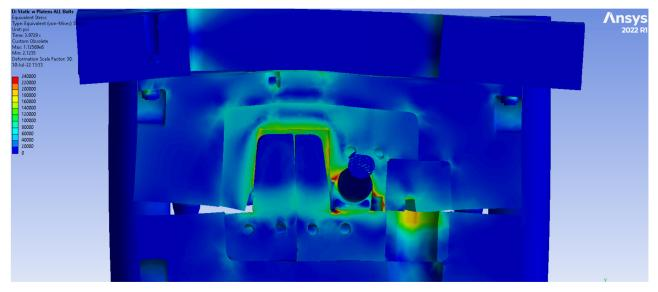
Stress plots on cavity inserts show hot spots on locations with thin walls, high thermal gradient, and geometric transition.
